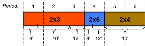
Figure 4: Production plan for a finishing line for six consecutive production shifts (periods).
